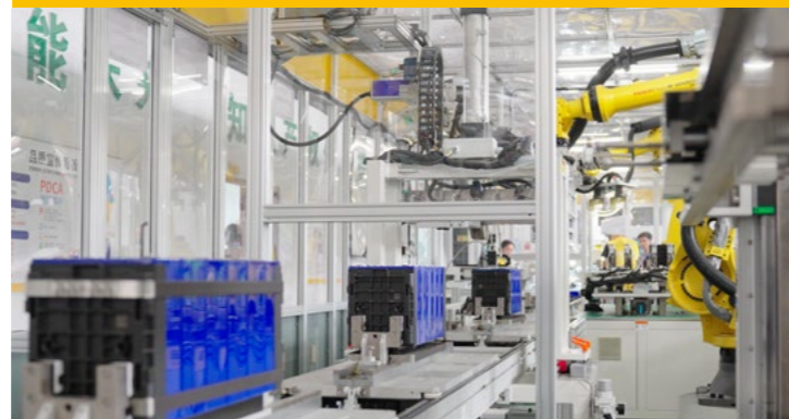
Automatic assembly line for battery cell modules (production site in Nantong)
