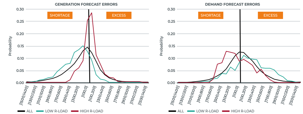
FIGURE 6-6 — PROBABILITY DISTRIBUTION OF DAY-AHEAD FORECAST ERRORS FOR GENERATION (LEFT) AND DEMAND (RIGHT) COMPARING ALL PERIODS 2020-21 (ALL) TO 1% LOWEST (LOW R-LOAD) AND 1% HIGHEST (HIGH R-LOAD) RESIDUAL LOAD PERIODS
