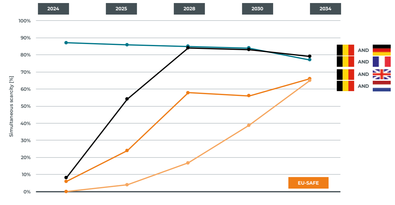
FIGURE IX-2 — SIMULTANEOUS SCARCITY EVENTS: BILATERAL SIMULTANEOUS SCARCITY BETWEEN BELGIUM AND EACH NEIGHBOURING COUNTRY (EU-SAFE SCENARIO)
