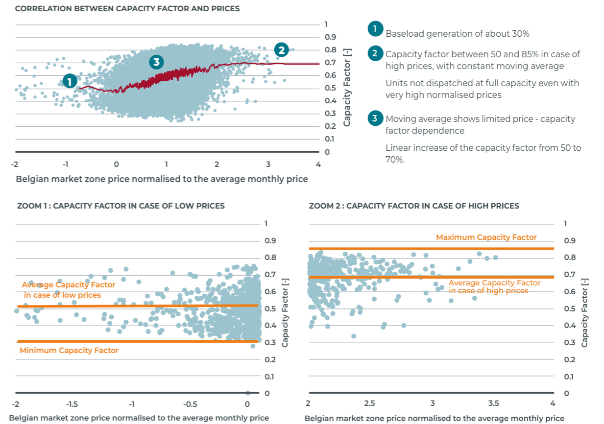
FIGURE C-5 — COMPARISON BETWEEN ELECTRICITY PRICES AND CAPACITY FACTOR OF SMALL/DSO-CONNECTED CHP UNITS (PROFILED UNITS) IN BELGIUM OVER 2018-2022
